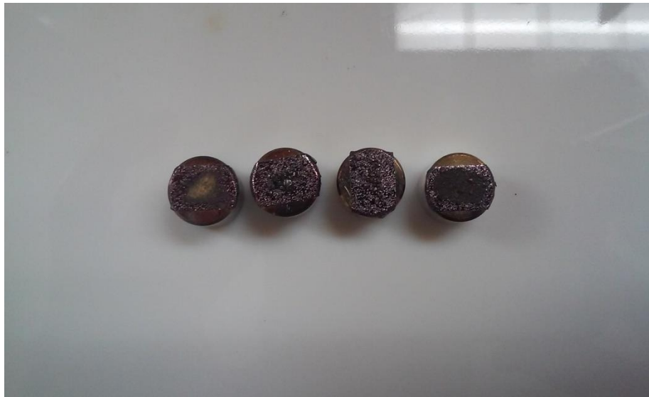
Samples coated with gold/palladium for SEM/EDS analysis
