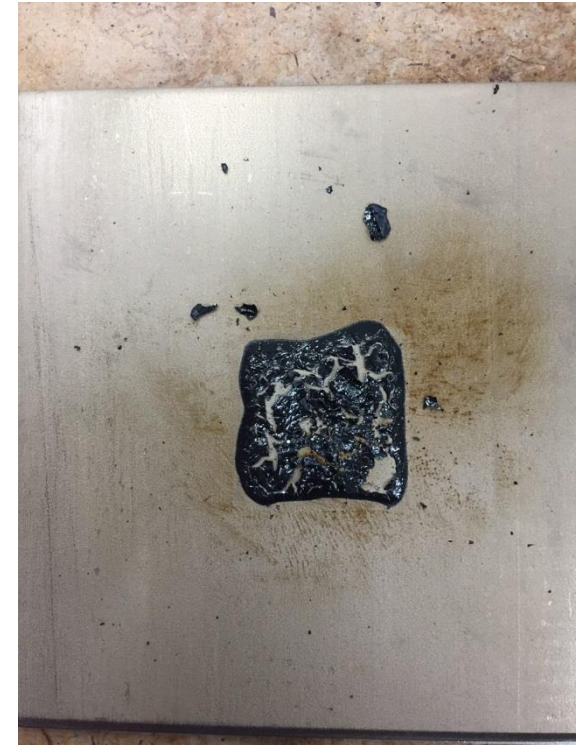
Significant mass loss, discoloration, desiccation, cracking, and flaking. Slightest abrasion with fixative resulted in total flaking. (800° F)
