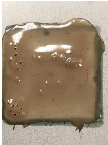
Discoloration, bubbling, continued expansion, “off gassing”, and mass loss (400° F)
