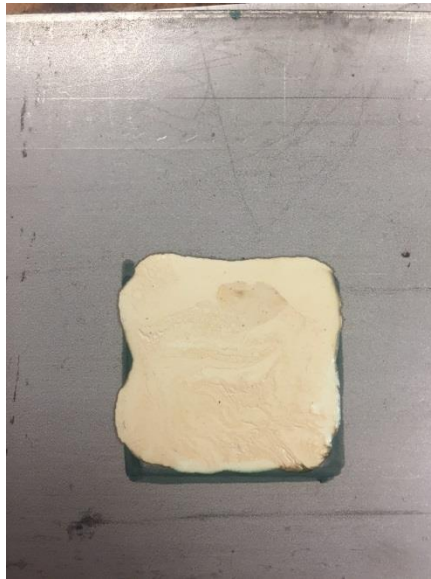
Discoloration, "off gassing", and mass loss (500° F)
