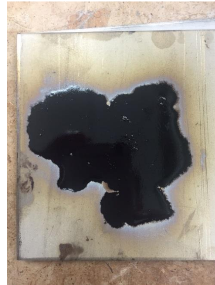
Significant discoloration, continued expansion and “off gassing”, mass loss, desiccation, cracking, and brittle composition (500° F)
