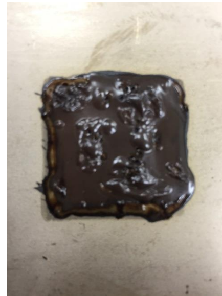
Significant discoloration, continued expansion, “off gassing”, mass loss, desiccation, cracking, and brittle composition (500° F)
