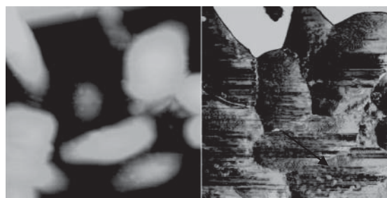
Figure 5F. G954 cultured in the media containing 0.5ppm uranium (scan size 3.89 \times 3.89 \mu\text{m}^2 ; Z range 250nm and phase angle 60^\circ ). Height and phase images clearly show precipitation on the cell surface.
